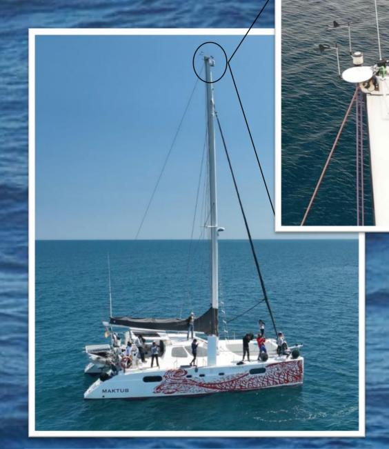
A FLIR M364C LR thermal camera installed on top of the mast of the Maktub, research vessel of the EDMAKTUB Association.
